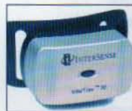
Sony's PLM-5700 (left) and the InterSense headtracker (above) together provide a hi-res virtual reality image that smoothly tracks head movement
